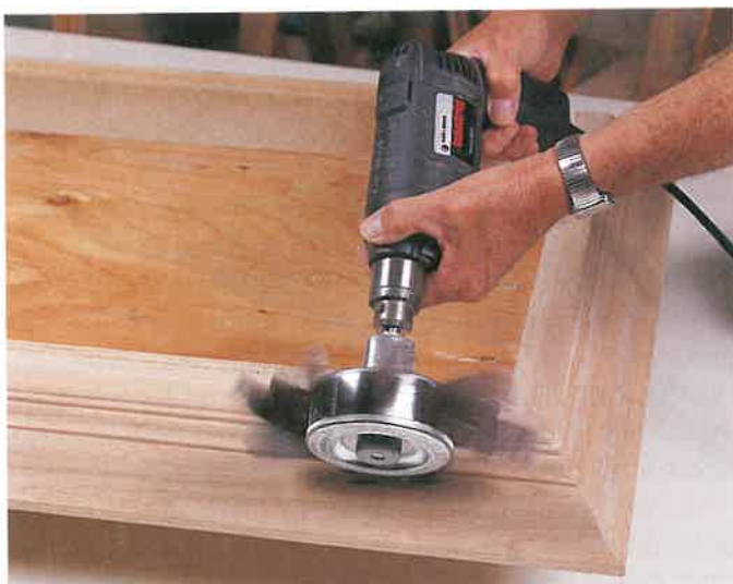
Figure 30-16. Flap wheels mounted on a drill will smooth in tight corners and around contours. (Chuck Davis Cabinets)
