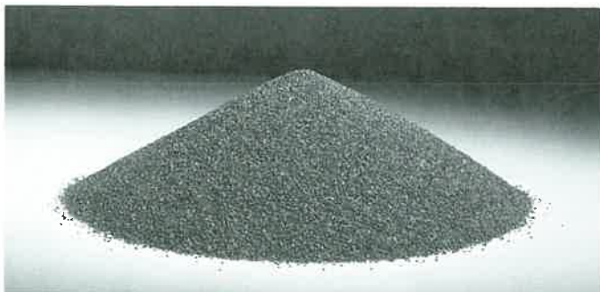
Figure 30-2. Abrasive grains are the essential ingredient for making solid and coated abrasives. (Norton)
