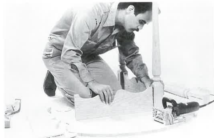
Figure 40-10. Assembling the legs and apron pieces using plate joinery. A—Mark slot locations on the legs. B—Mark slot locations on the apron pieces. C—Cut the apron slots. D—Align the apron and leg to cut the leg slots. E—Put glue and a plate in both slots on one leg. F—Assemble the legs and apron on a flat surface. (Steiner-Lamello)
