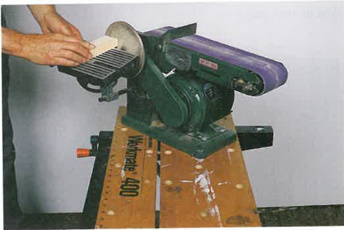
Figure 31-13. By using a miter gauge and a tilting table, many different workpieces can be abraded. (Delta International Machinery Corp.)
