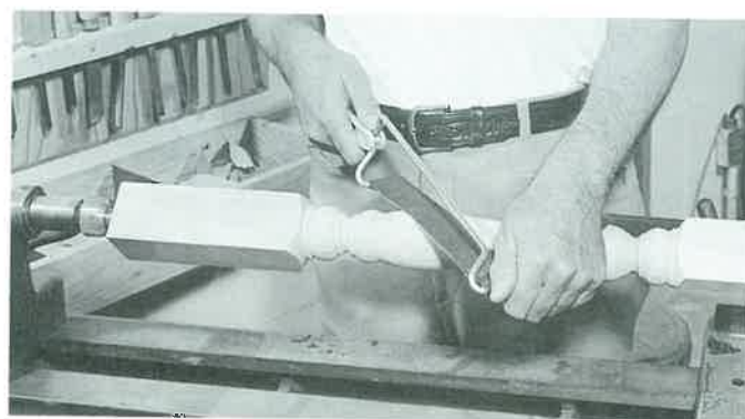
Figure 31-7. A—Make a contour block to sand moldings, trim, and other curved surfaces. B—Strips of abrasive used by hand or in a bow sander work well with turned pieces. (Glit, Inc.)
