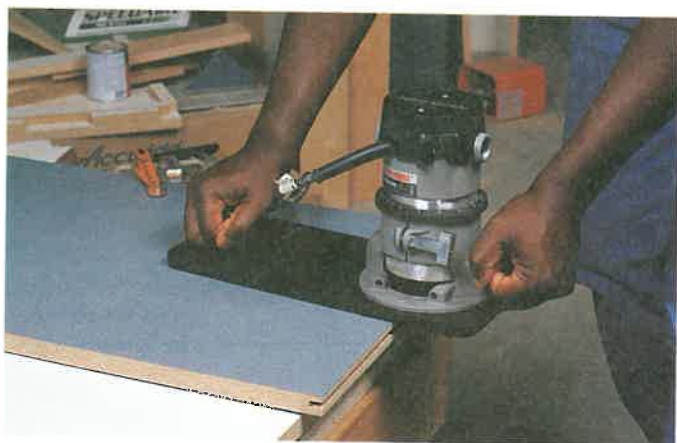
Figure 36-10. A—This router is fitted with a wide base and 3-wing slot cutter. B—Hold the router steady, and firmly move it along the panel. ( Chuck Davis Cabinets )
