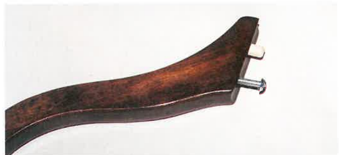
Figure 40-16. Place an insert nut and dowel in the leg. The screw travels through the pedestal and threads into the insert nut.
