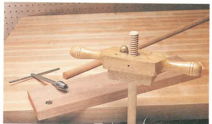
Figure 29-76. Making threaded joints. The die produces external threads and the tap produces internal threads. (American Machine & Tool Co.)
