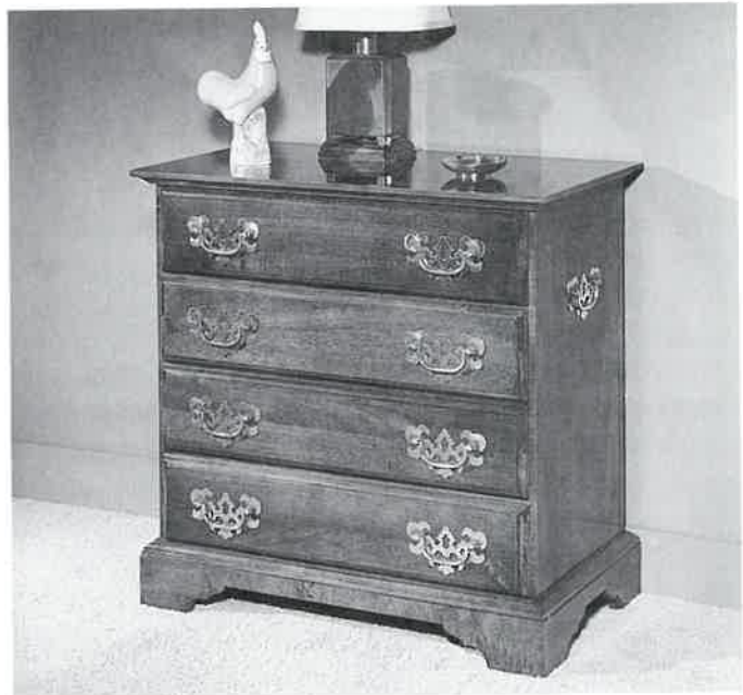
Figure 40-1. Each flat bracket foot consists of two parts joined with a reinforced miter joint. Here the edges are shaped for appearance. ( Mersman Tables )
