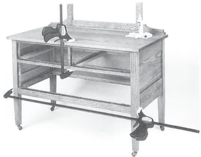
Figure 33-1. Clamps are placed on the workpiece after the adhesive is applied ( American Tool Companies )
