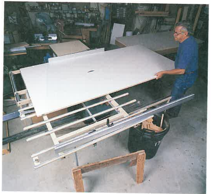
Figure 38-22. This table saw is equipped with accessories that permit handling large panels. (Chuck Davis Cabinets)
