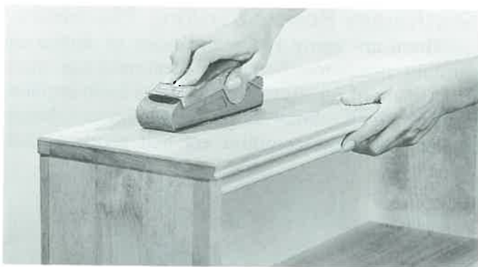
Figure 31-5. Sanding along the wood grain makes abrasive scratch marks less visible. (Norton Co.)
