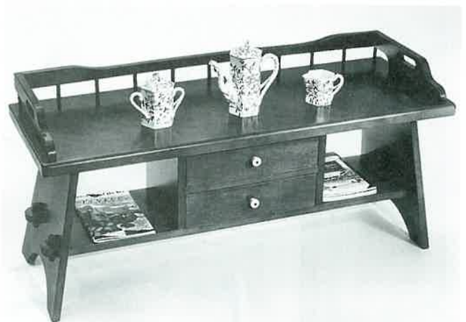
Figure 29-47. Tusk tenon on an Early American coffee table. ( Craft Products )
