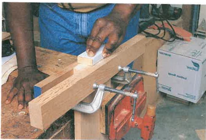
Figure 31-6. Use C-clamps to secure scrap wood when sanding end grain.
