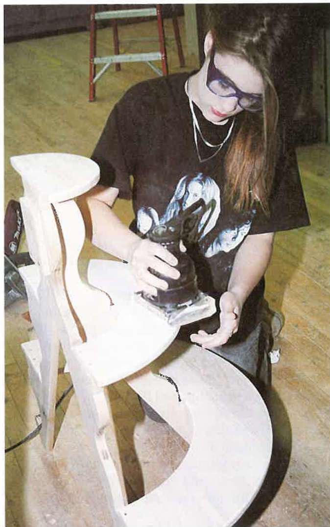
Figure 30-1. Abrasives are used to smooth workpieces before finishing. (Montachusett Regional Vo-Tech School, Fitchburg, MA)
