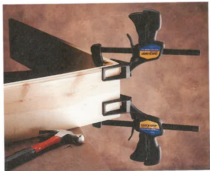
Figure 33-6. Clamps can secure mitered corners. (American Tool Companies)
