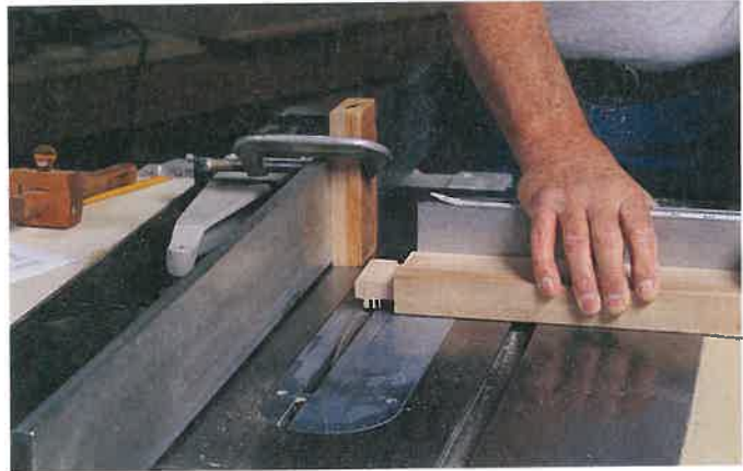
Figure 29-43. Sawing tenons by making a series of crosscut passes. Guard was removed to show process ( Chuck Davis Cabinets )
