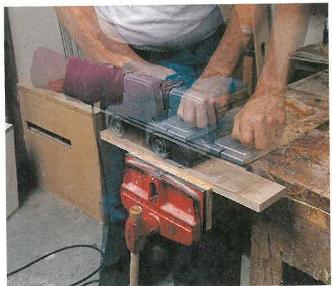
Figure 31-23. Move the belt sander in short overlapping strokes. Check the tracking for proper adjustment before and while using the tool. (Chuck Davis Cabinets)
