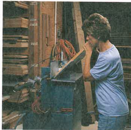
Figure 29-63. Stationary plate joiner. A—Cutting kerfs in the edge of a base cabinet bottom panel. B—Using a standard accessory to cut kerfs for a miter joint. C—Cutting kerfs in the side of a cabinet side panel. (Chuck Davis Cabinets)
