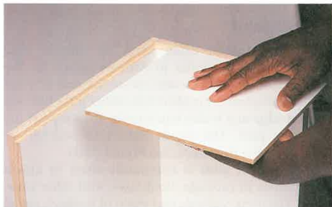
Figure 29-12. Rabbet joints are often used to hide the back panel edge and end grain.
