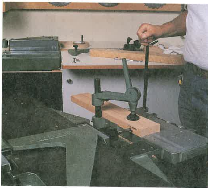
Figure 29-30. The horizontal boring machine provides a movable platform for creating the mortise. ( Chuck Davis Cabinets )
