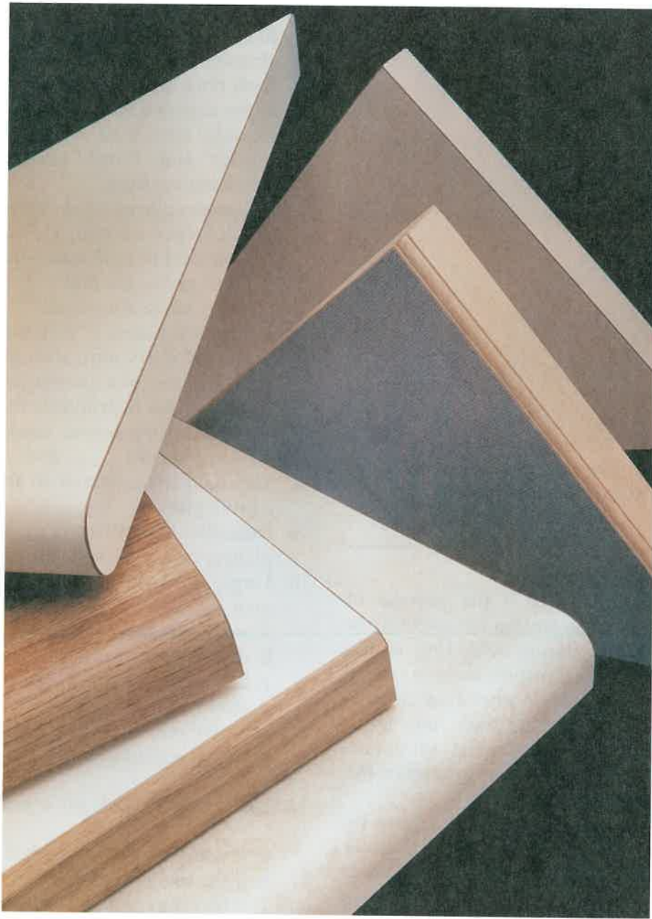
A solvent-base contact cement was used to bond the plastic laminates to the various workpieces.
