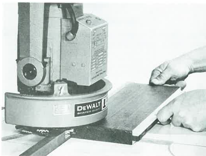
Figure 29-26. Cutting the groove with a radial arm saw and dado blade. (DeWalt Industrial Tool Co.)
