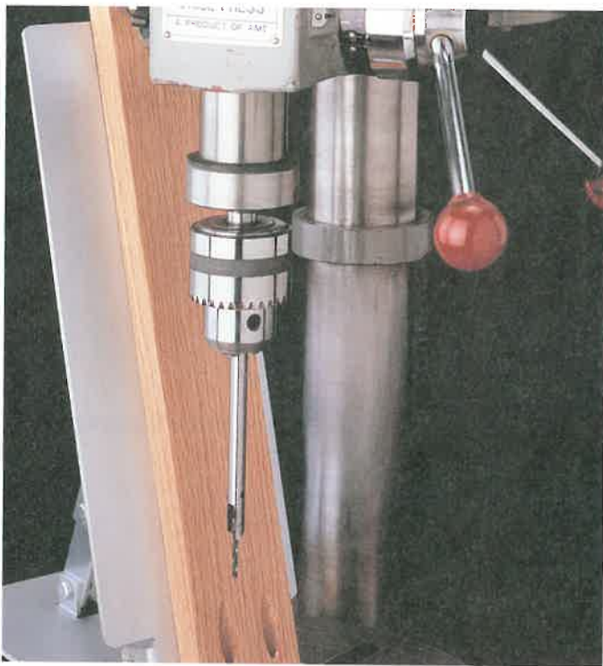
Figure 29-72. Jig for making pocket joints. (Portalign Tool Corp.)
