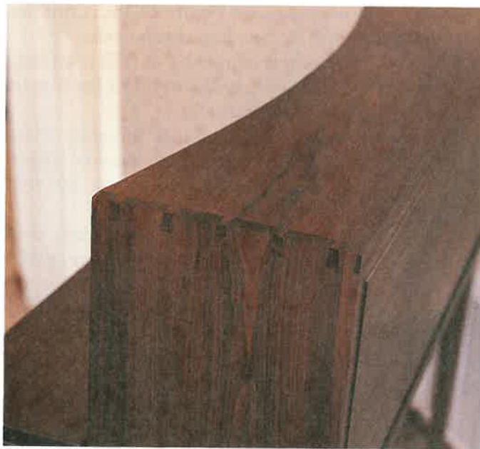
Figure 29-49. Dovetails are an intricate, but attractive joints. Through dovetails are similar to half blind dovetails. The end grain of both the pin and the tail are visible and may be decorative. (Chuck Davis Cabinets)
