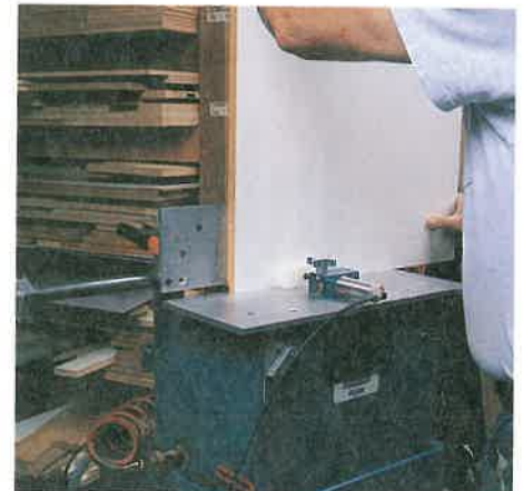
Figure 29-63. Stationary plate joiner. A—Cutting kerfs in the edge of a base cabinet bottom panel. B—Using a standard accessory to cut kerfs for a miter joint. C—Cutting kerfs in the side of a cabinet side panel. (Chuck Davis Cabinets)
