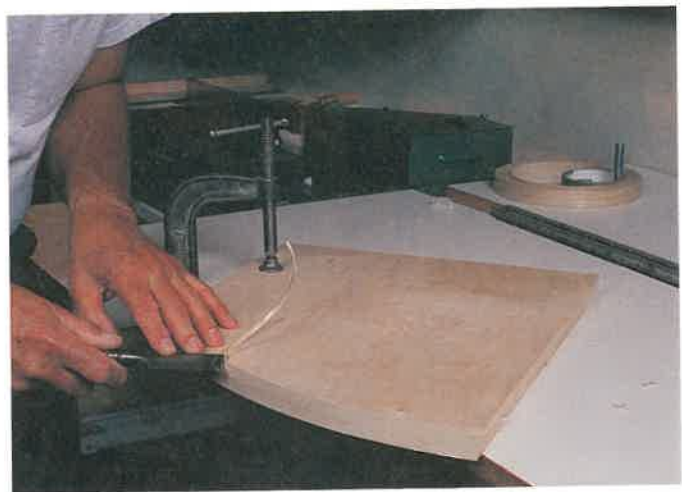
Figure 35-12. Trim tape on curved edges with a sharp chisel. ( Chuck Davis Cabinets )
