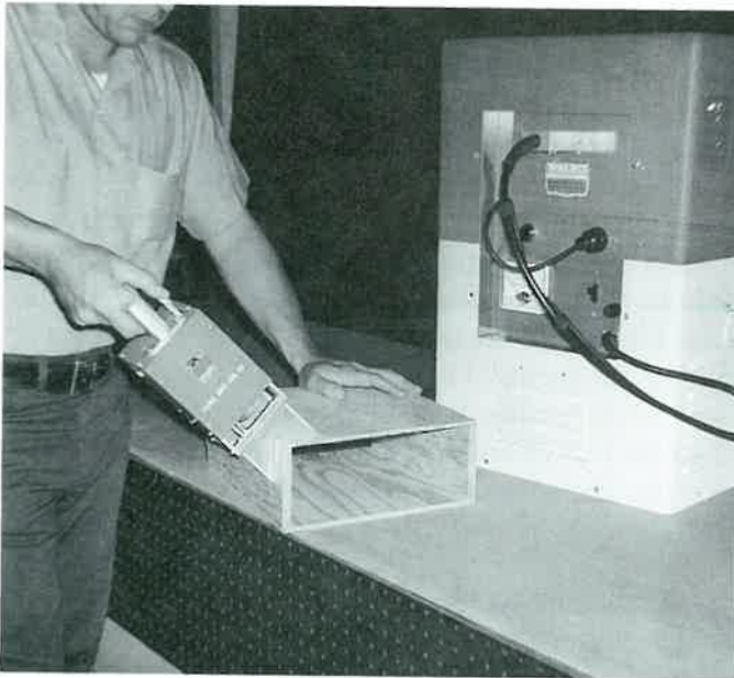
Figure 32-22. Large scale RF gluing machines clamp the stock. Here, a 15 piece face-to-face lamination is being RF glued. ( Mann-Russell Electronics )
