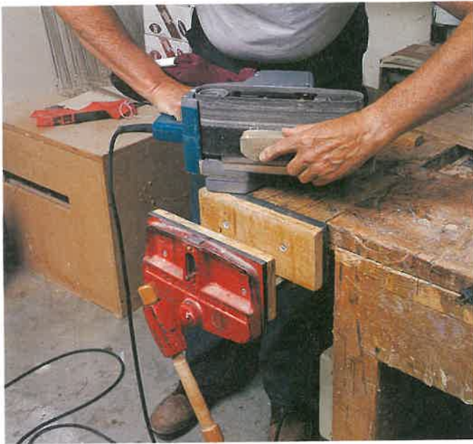
Figure 31-35. A rubber-like cleaner removes resin and chips from abrasives. (Chuck Davis Cabinets)
