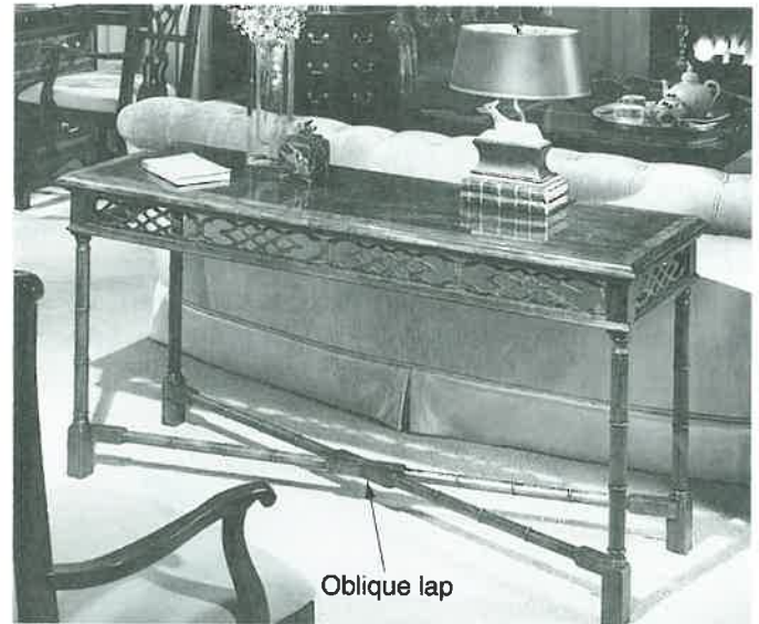
Figure 29-19. The oblique lap connects stretchers at their intersection. (Thomasville)
