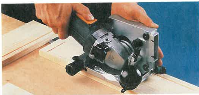
Figure 29-58. Using a portable power plate joiner to prepare components of a drawer for assembly. (Black & Decker)
