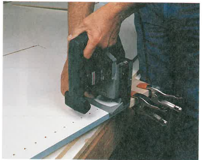
Figure 29-64. Use a portable plate joiner to cut kerfs away from the edge of the panel. (Chuck Davis Cabinets)
