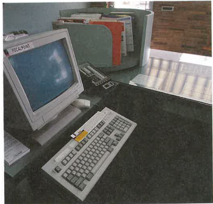
Figure 36-22. This lazy Susan has substrate of KerfKore®. The process is similar to making a radius door. ( Chuck Davis Cabinets )
