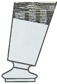
Figure 40-39. Shown is a leg ferrule with a glide.
