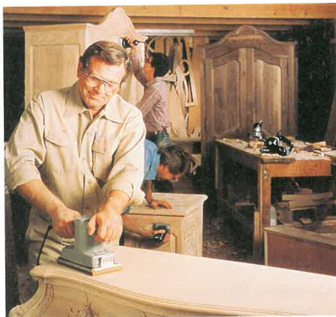
Figure 31-1. This assembled product is abraded with an in-line sander before applying finish. (Porter-Cable Corp.)
