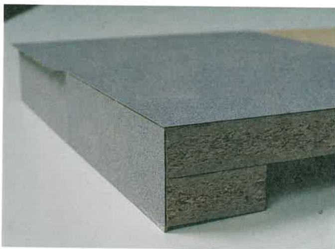
Figure 36-6. Surface laminate overlaps the edge banding that was applied first. The trimming is not complete to show the overlap. The 3/4" (19 mm) build down blocking is for appearance. It makes the tabletop look thicker. (Chuck Davis Cabinets)
