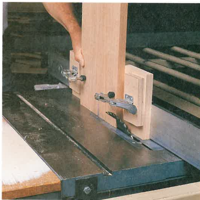
Figure 39-14. Beveling the panel on the table saw. (Chuck Davis Cabinets)
