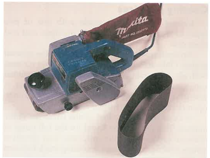
Figure 30-12. Abrasive belts are used on portable belt sanders. (Chuck Davis Cabinets)
