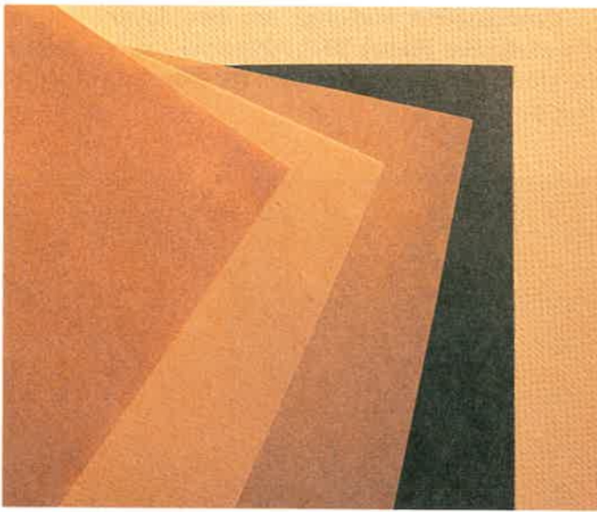
Figure 30-4. Types of abrasive paper (from right to left): Silicon carbide (blue black), aluminum oxide (tan), flint paper (light tan), and garnet paper (reddish brown).
