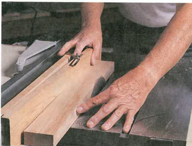
Figure 40-17. Make a taper jig to cut tapered legs. Let in a cleat to act as a push stick. The guard was removed to show the operation. (Chuck Davis Cabinets)
