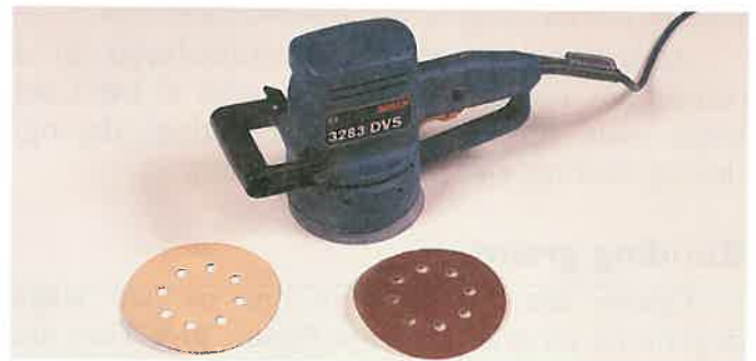
Figure 30-13. Disks for portable power random orbital sanders are punched with several holes to facilitate dust removal. (Chuck Davis Cabinets)
