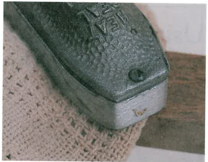
Figure 31-2. Raise dents with steam created by applying a hot hand iron to a damp pad before abrading. (Chuck Davis Cabinets)
